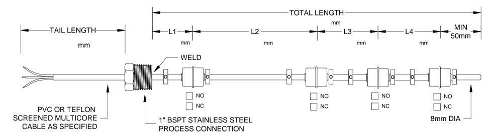
STANDARD - NO or NC CONTACT RATED AT 32V AC/DC @ 500mA RESISTIVE LOAD
